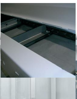
Coolant and chips flow from the machine into the watertight frame of the Turbo MS500. Filter boxes, strategically located along the conveyor load section, allow the coolant to escape into the machine tank providing 500 micron filtration. Brushes attached to the conveyor's scraper bars provide a self cleaning method to wipe contaminants from the boxes as the conveyor belt advances.
