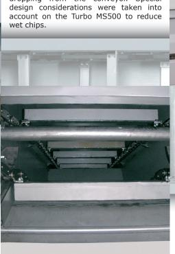
normal conveyor operation. Coolant flow and optimal filtration is assured, as the design of the Turbo MS500 allows the number of filter boxes used to be matched to the requirements of the machine tools maximum flow rate.
