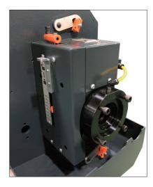
The upgraded front rest with universal V-shaped guiding elements adapts to any round bar diameter, dampening any residual vibration and noise within the whole diameter range. Hexagonal and profiled bars will greatly benefit from the optional O-shaped guiding elements to reach the optimal performance.
