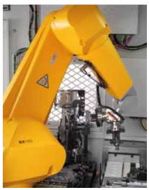
Double gripper head, Post-process gage, SPC and reject drawers
