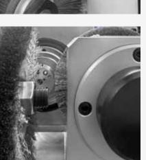
Simultaneous face and outside diameter brush deburring
